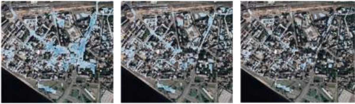
Figure 5-7. Modelling various scenarios in a surface runoff flooding model
